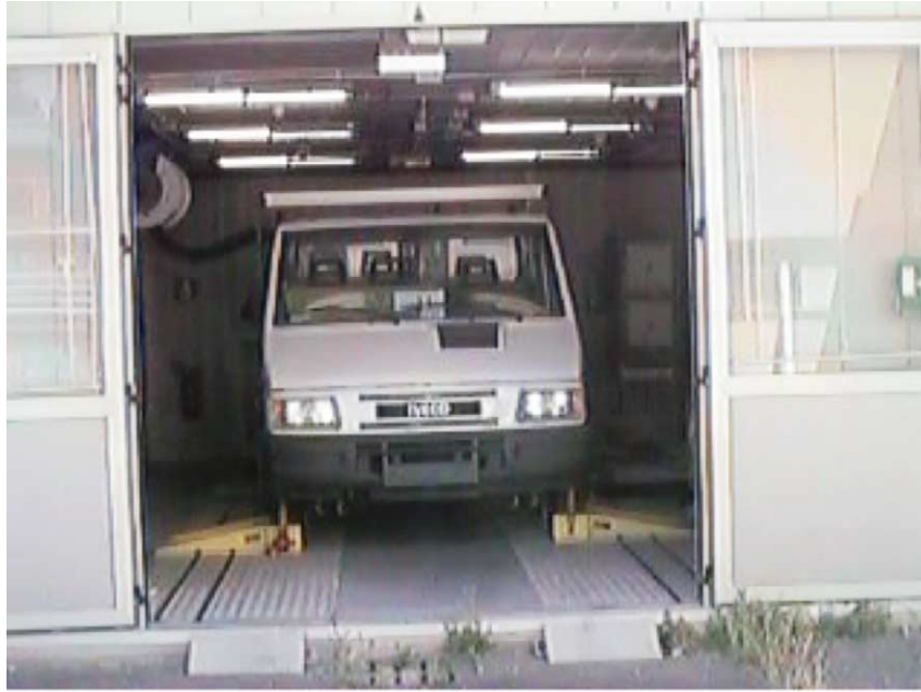
Fig. 5. Picture of the roller bench test facility at ENEA Casaccia Research Centre.
