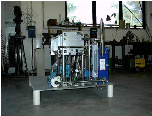
Fig. 11. The 35 kW prototype of a triple hybrid (FC + UC + battery) jointly developed by ENEA and University of ROMA TRE.
