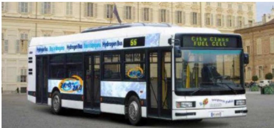
Fig. 2. Irisbus hydrogen-fueled, FC powered bus operating in the city of Turin.
